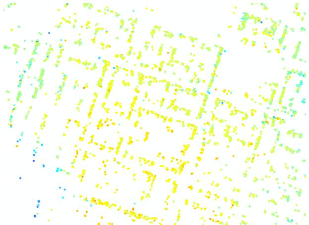
Figure 12. Atmosphere phase shift for Aug. 21<sup>st</sup>, 2008 based on TerraSAR-X PSI data (same area as Fig. 11)
