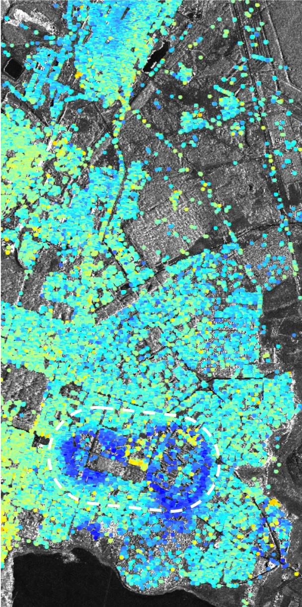
*Figure 13. Slight TerraSAR-X PSI derived atmospheric phase shifts for September 1<sup>st</sup>, 2008 in Berezniki. White dashed ellipse emphasizes main deformation area*
