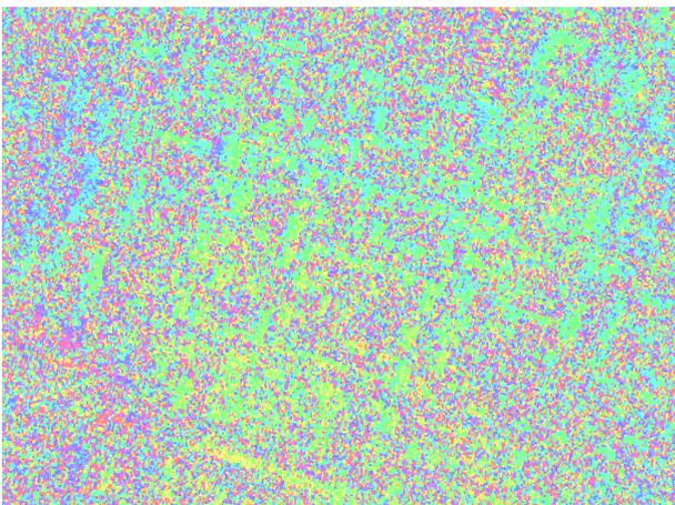
Figure 11. Atmosphere phase shift for Aug. 21<sup>st</sup>, 2008 based on TerraSAR-X DInSAR data (Berezniki area)
