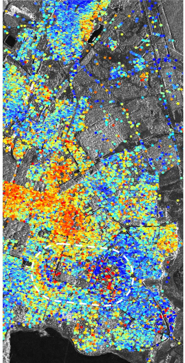
*Figure 14. Strong TerraSAR-X PSI derived atmospheric phase shifts for August 30<sup>th</sup>, 2009 in Berezniki. White dashed ellipse emphasizes main deformation area*
