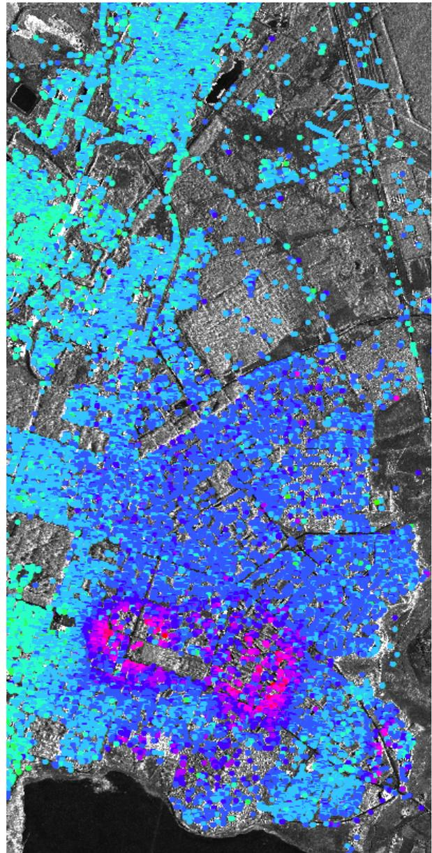
Figure 15. TerraSAR-X PSI result for mean deformation signal computed from unwrapped atmospheric signals. Left side of image shows no deformation (cyan), whole lower right part of Berezniki shows slight subsidence. Boundaries of higher deformation areas are clearly visible, though inner parts were not correctly represented due to phase ambiguities in the averaging process (cf. also chapter 2 for details)
